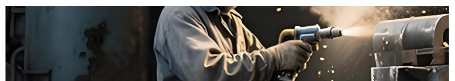
Sandblasting uses high-speed abrasive (e.g., sand) to impact the metal surface, removing rust, dirt, and oxides, while creating a rough matte effect that enhances the adhesion of coatings.
