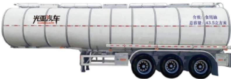
Aluminum Alloy Edible Oil Transport Semi-trailer
