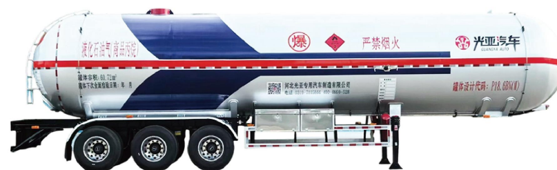
60.72 m 3 LPG (Commercial Propane) Transport Semi-trailer
