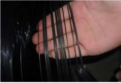
Black annealed wire is a wire that has been heated and cooled to give it a black appearance. It has certain toughness and corrosion resistance and is suitable for various industrial and construction fields.
