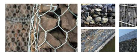
Gabion mesh is a mesh structure woven from galvanized or PVC galvanized steel wire. It is usually used in earth and rock engineering, river protection, environmental management and other fields. It has a simple structure and is easy to install. It can effectively prevent soil and rock collapse, bank protection, and slope protection. It has good water permeability and is widely used in various civil engineering projects.
